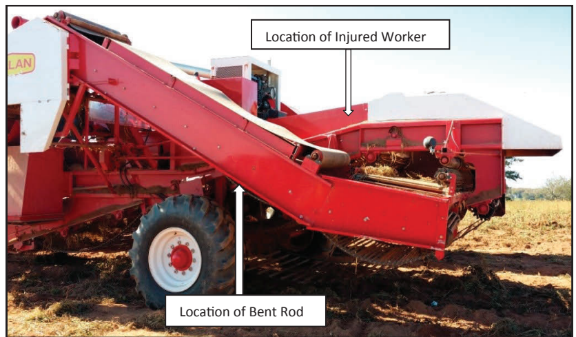
Figure 1. Location of bent rod and injured worker on the potato harvester
