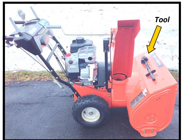
Figure 3. Common household snowblower with chute-clearing tool attached.
